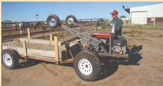
Instead of towing a wagon or other trailing equipment, Mark Lyon's unusual looking single axle tractor actually "self-propels" whatever it's hitched up to.
