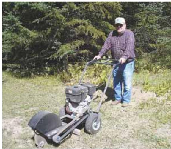
Ron Mickle built this stump grinder that rides on 10-in. pneumatic tires and is powered by a 13 hp. Briggs & Stratton engine.
