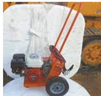
To provide portable 12-volt power, Steven Zook married a 4 hp. Honda engine to an alternator and mounted it on a 2-wheel push cart.
