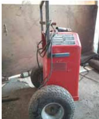
holes on back of the welder serves as an axle."
