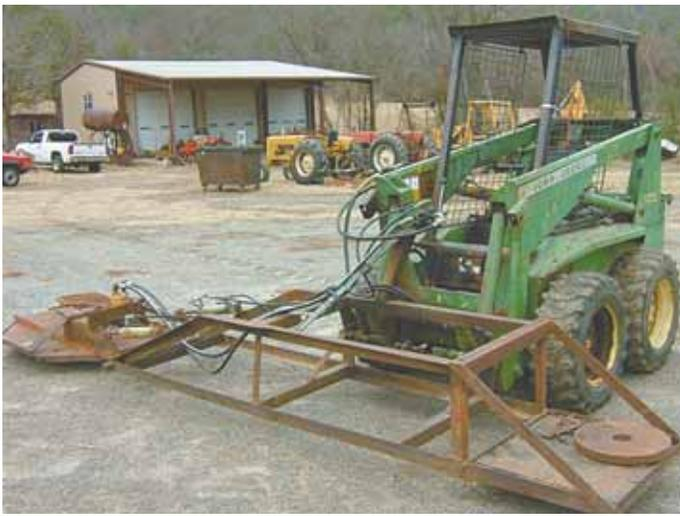
Allen Kimball uses his skid loader-mounted rotary mower to keep roadsides well mowed. A carrier rack with counterweights on the opposite end lets him get into tight-places.
