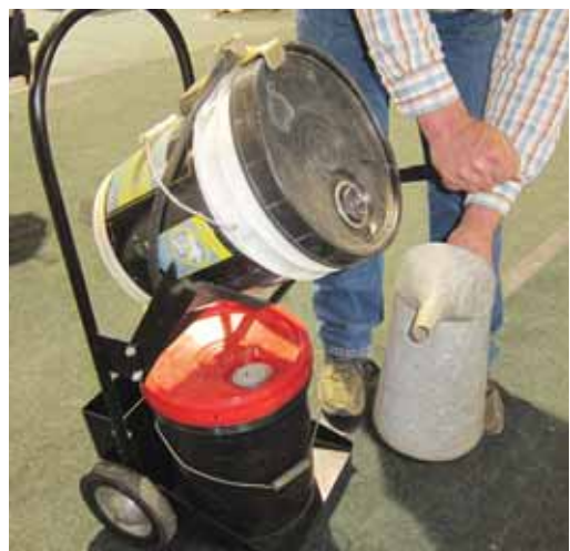
Pail Tender lets you easily control the pail with one hand and hold the container you're pouring into with the other.
