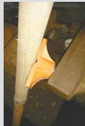
Gyrojaw is a pyramid-shaped attachment that fits against the jaw of a standard bench vise. It's designed to clamp uneven objects.
