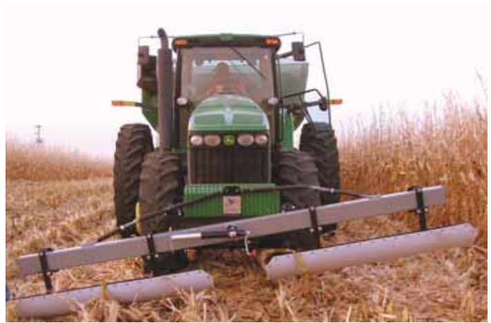
Unit pivots in the middle to stay in contact with the ground at all times on uneven ground. A pair of heavy duty springs bring it back to the neutral position.
