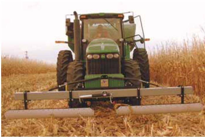
Tractor-mounted "Stalk Punisher" flattens corn stalks across entire width of tractor. Two 6-ft. long skids that clamp onto a toolbar can be moved in or out.
