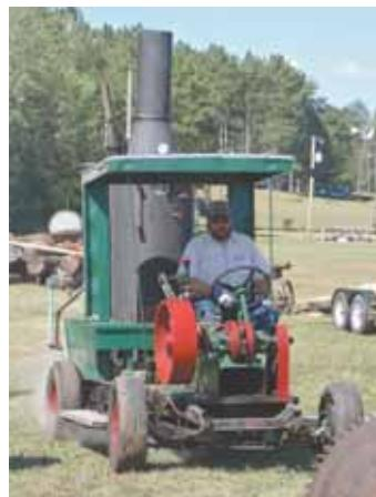
David Brazeau created this steam-powered car, putting the boiler in back and the steam engine in front.
