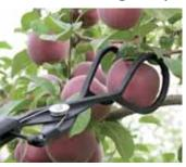
"Twister Fruit Picker" is designed to screw onto a standard threaded pole so you can stand safely on the ground.
