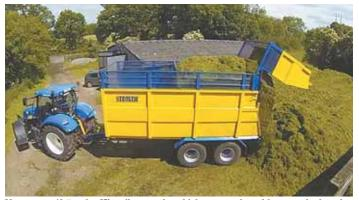
Kompactor 40 "push-off" trailer travels at highway speeds and has a push plate that serves as a compactor when the trailer is being loaded in the field. The box can be quickly removed so the trailer frame can be used for more than one job.
