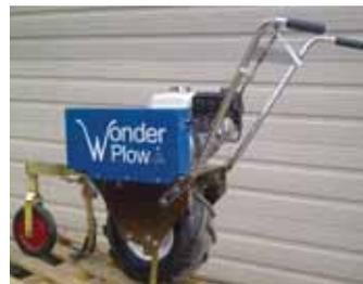
**You can use the self-propelled Wonder Plow as a plow, cultivator, seeder, or fertilizer unit, eliminating the need to buy separate machines.**
