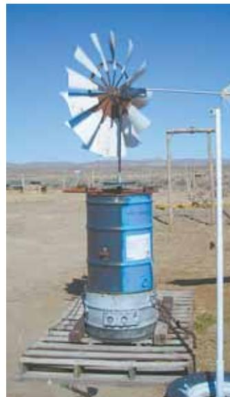
**Jeff Hoard, an off-grid inventor, makes chicken mash with homemade equipment including this wind-powered alfalfa mill (left) and a modified flour mill.**
