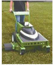
Walk-behind, 33-in. wide electric mower runs on a lithium energy module power pack.
