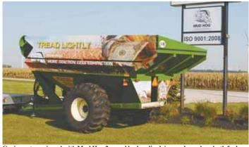
Grain carts equipped with Mud Hog 2-speed hydraulic-driven axles reduce both fuel use and compaction, says an Indiana company that offers the axle drive on J&M grain carts.
