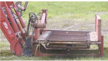
Edgar used unloading chain from a forage wagon to make unloader.
