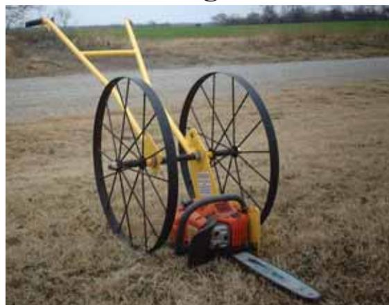
"Chainsaw Caddie" provides a way to hold and maneuver a chainsaw close to the ground, so you don't have to bend over, stoop or carry the chainsaw.
