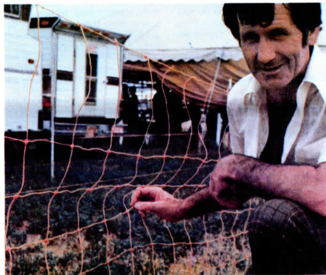
Any conventional electric charger used for regular single-wire electric fence can be used to “charge” Flexinet electric netting.
