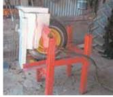
mounting a wheel hub and tire on a metal frame (above). Homemade cracker (below) is fitted with a 10-in. long bolt that has a 4-bladed knife screwed onto the bottom.
