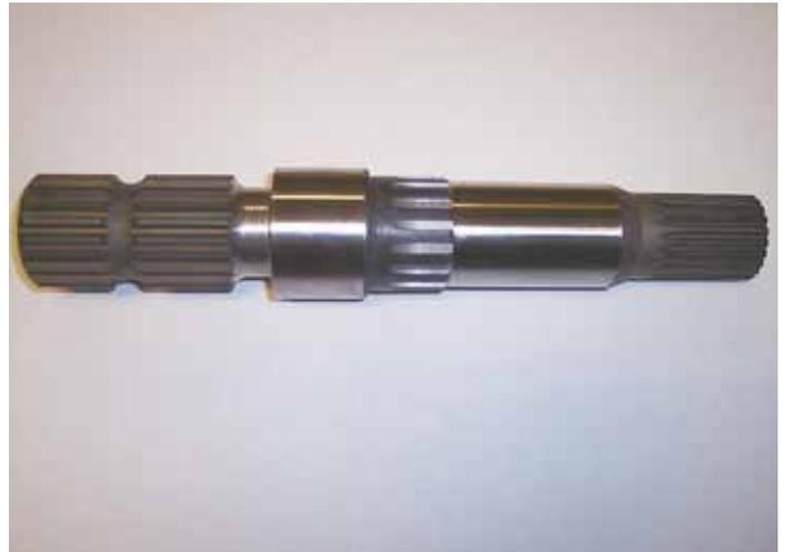
Insert shaft makes it easy to hook up an older Deere tractor to a mower or some other tool with a 20-spline pto shaft.
