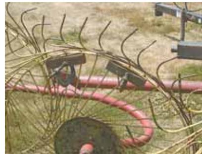
Jim Brashears says using 4-in. C-clamps and wooden blocks makes it easy to replace broken teeth on his wheel hay rake.
