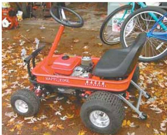
"Hot rod" Radio Flyer is powered by a 6 1/2 hp Honda clone engine.
