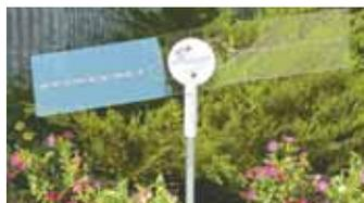
Clear plastic blade is fitted with 18 multi-colored LED lights connected to a generator. Wind spins blade to power the generator to light the LED's.
