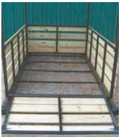
Hinged gate on front of feeder lowers to the ground, allowing Prewett to roll bales up the ramp by hand.
