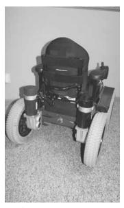
Sullivan bought 4 quality wheels off eBay and uses 4 motors to run them independently. To reduce weight, he made a compact aluminum frame just big enough to hold the motors and wheels.
