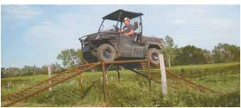
Drive-over gate comes with a 5-ft. long table and two 14-ft. long, 6-ft. wide ramps that bolt onto table. Bolts run through sleeves, allowing ramps to flex up or down.
