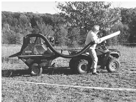
**Sam McNair's homemade, tow-behind vacuum turns horse manure into a fluffy, dry material that's ready to compost.**
