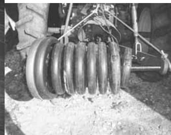
A wide variety of adapter kits are available, allowing you to mount weights on a tractor’s drive wheels or on the front, back or sides of the tractor.
