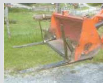
Raube McDaniel built bucket-mounted log forks for his 2007 Kubota B7510 loader tractor, bolting the leaf springs from a 3/4-ton pickup to the sides of the bucket.
