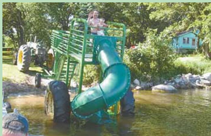
A hitch on front allows Seifert to back the big rig down into a lake using a real Deere tractor. A sump pump brings water up to top of slide to make it slippery and fast.
