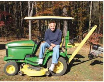
Bobby Milam's winch-operated boom is shown here lifting a power generator that weighs about 80 lbs.
