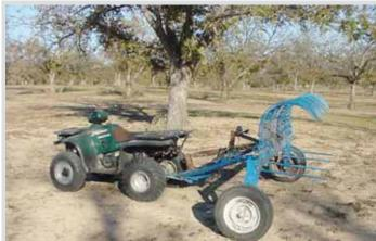
Lightweight "stick rake" is used after pecan trees have been shaken. Tines are raised and lowered by an electric screw cylinder.
