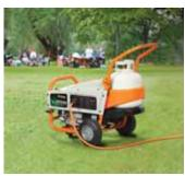
Built-in 20-lb. LP tank holder on Generac generator eliminates the need to carry the tank separately.
