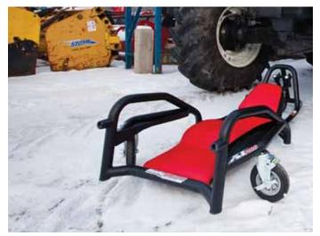
The frame on this heavy duty floor creeper is built strong enough to withstand the weight and impact of a falling vehicle.
