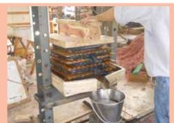
The shredded apple pulp is put into Miller's 24-in. square press made from oak and lined with stainless steel.
