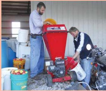
Apples are dumped into a Troy Bilt brush shredder, with the shredded pulp and juice discharged into a 5-gal. pail.
