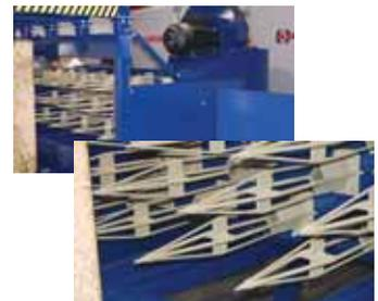
"Spears" inject heated air into bales.
