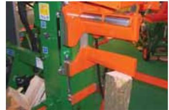
Rollers on 2-part splitting wedge keep wood from binding up on return stroke.
