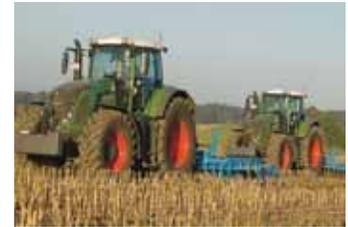
Automated controls allow driver in front tractor to control second "slave" tractor that follows behind.
