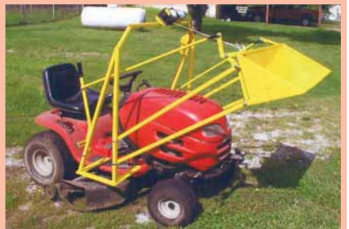
Home-built bucket is raised and lowered by a 12-volt electric winch that’s operated by a 2-button remote control.
