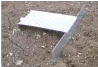
Water flows over built-in dam, through screen, and into box and pipe underneath.
