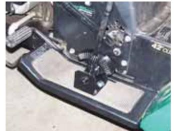
He removed the pitman shaft and gear sector, as well as the steering gear, and remounted them outside above the footrest.
