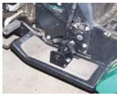
He removed the pitman shaft and gear sector, as well as the steering gear, and remounted them outside above the footrest.
