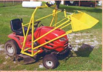
Home-built bucket is raised and lowered by a 12-volt electric winch that's operated
