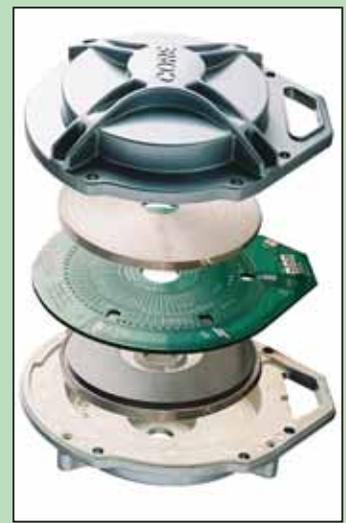
**Conductor Optimized Rotary Energy (CORE) motor eliminates wound wire and other complexities of conventional electric motors. Exploded view of motor (above) shows printed circuit board with embedded wires sandwiched between two permanent magnet rotors. The first outdoor tool with a CORE motor - a weed trimmer - will be introduced this spring.**
