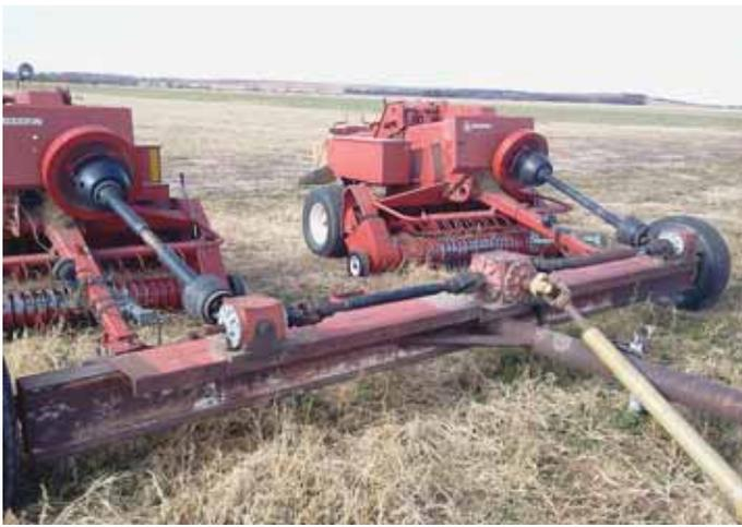
Dale Hanson's 2-wheel hitch lets him pull 2 balers at one time, at nearly half the cost of a commercial 2-baler hitch.
