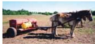
Modified grain drill allows Floyd Summy to plant corn in 15-in. rows. gal. per acre."
