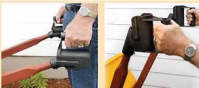
Pivoting handles fit onto wheelbarrow's existing handles, allowing you to lift and dump a load without having to reposition your hands.
