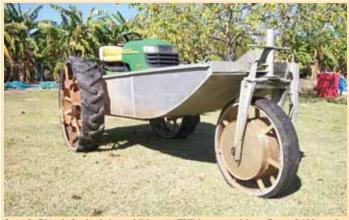
Jesse LeBlanc's 3-wheeled amphibious "ATV" is powered by a Deere L100 garden tractor that rides inside a homemade, 10-ft. long aluminum boat.
