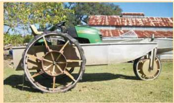
Rig's 4-ft. high aluminum rear wheels are lined with rubber lug treads. Inner hubs support a series of 8-in. long metal paddles that help propel boat through water.
