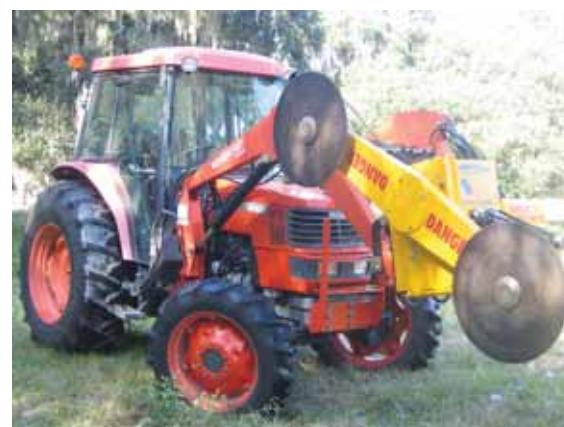
"ChopZilla" attachment for tractors and skid loaders uses two 24-in. saw blades mounted on a rotating 7-ft. beam.
