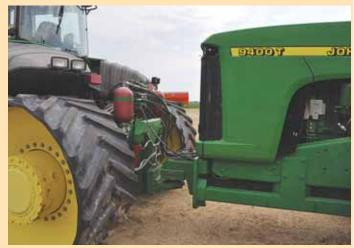
Hitch system between tractors uses a pair of hydraulic cylinders and accumulators to dampen up and down movement. A hitch frame runs back to the drawbar on the rear tractor. It's braced to the rear tractor frame with steel plates.
