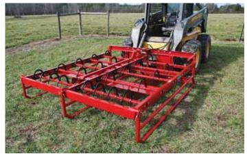
Loader-mounted "Accumagrapple" gathers up 8 to 10 small square bales in the field. It eliminates the need for a separate accumulator.
