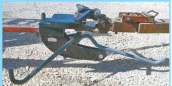
"Slick Hitch" consists of 2 parts – a curved unit that mounts on tractor drawbar and has a long "tail" rod bolted onto it that's free to swivel up or down, and a set of V-shaped metal rods spaced about 26 in. apart.
