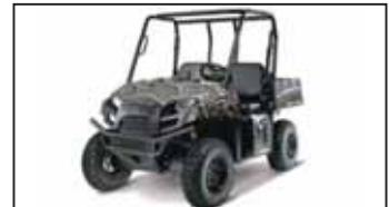
powered by a 30 hp, 48-volt high efficiency AC-induced electric motor and comes with eight 12-volt batteries. It also comes with its own recharger that plugs into a standard 110-volt AC outlet. The company says it'll go 50 miles on a single charge. I recharge it every night so I never run out of power."
