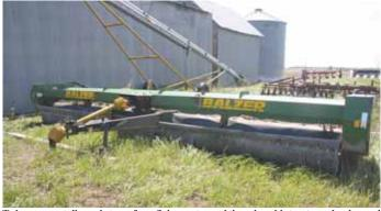
To keep corn stalks and stones from flying up toward the cab on his tractor as he chopped stalks, Harold Fratzke bolted a 2-ft. deep length of grain conveyor belting across the front of his Balzer stalk chopper.
