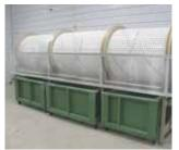
Nuts drop down through 2 sets of lawn mower tires that run at different speeds to "rub" hulls off (left). Nuts are then fed into a home-built sorting machine.
