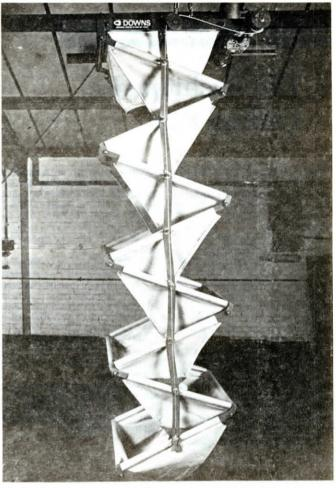
The Zig-Zag chute automatically unloads up to 60 tons of potatoes per hr. from a height of over 8 ft. Crop is gently "walked" down in zig-zag fashion to prevent damage. As pile height increases, the chute retracts up within itself without restricting flow of material.
