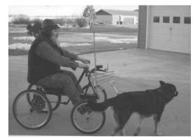
Split axle cart is fitted with a homemade "eccentric" drive on one side that's powered by pumping on a T-handle. A big dog can also be used to pull the cart.
