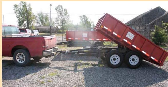
Operator sets the trailer brakes and then backs up. As upper frame and trailer box slides back past end of lower frame, it dumps.
