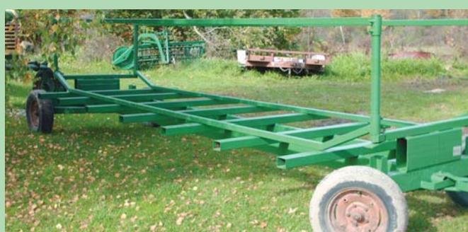
Portable round bale feeder is built on a used wagon running gear and has room for two rows of 3 bales.
