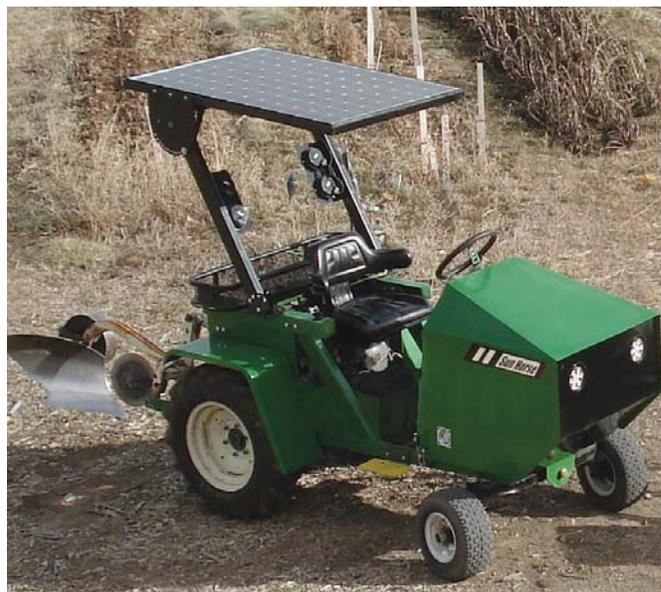
Sun Horse electric tractor can do several hours of light work before it needs recharging, or it can be used to power AC tools.
