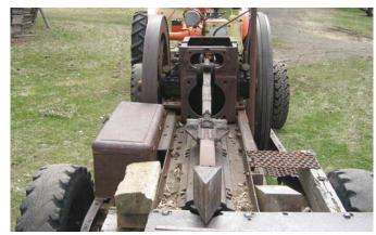
Splitter was built using the engine block, crankshaft and flywheels from a 1908 Mogul
