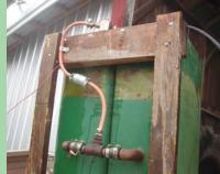
McAlister bolted together two fuel tanks off an old Oliver combine (left). He plumbed the tanks together with a T fitting and hose that goes to an electric fuel pump.
