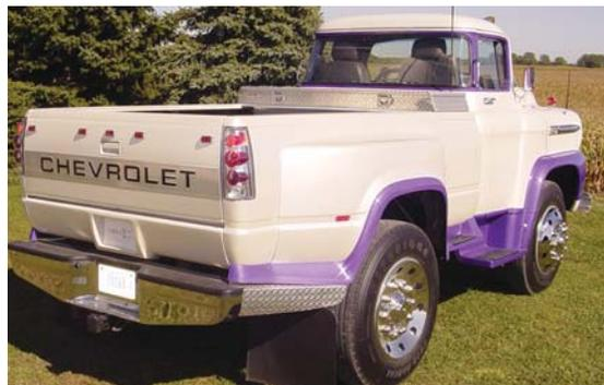
Les Miller made this big pickup by replacing the grain box on a 1959 Chevy straight truck with a 1989 Chevy dually bed.
