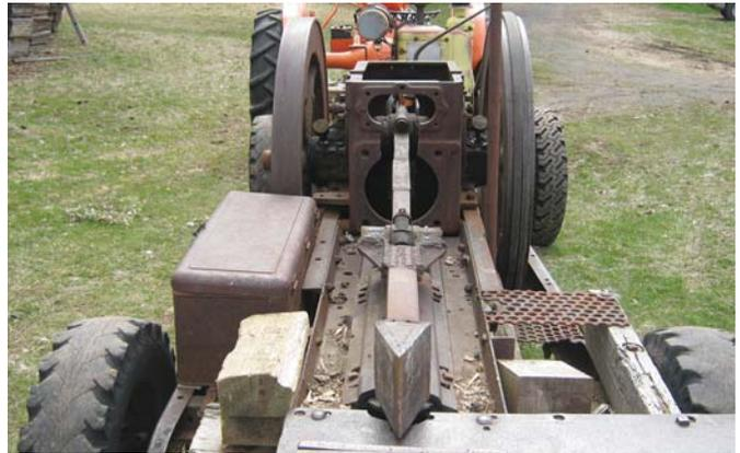
Splitter was built using the engine block, crankshaft and flywheels from a 1908 Mogul 8 hp tractor.
