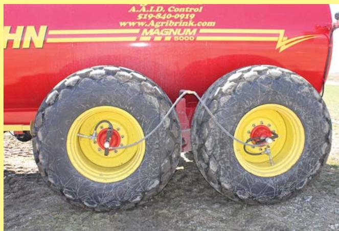
Automatic Air Inflation/Deflation system allows you to adjust your implement's tire pressures with the touch of a button.
