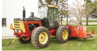
Virgil Poock and son Travis reversed the mounting brackets and drive system on their pull-type windrow merger so they could push it rather than pull it.
