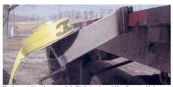
Hand-operated "ratchet strap winder" is designed to quickly roll up round bale straps. It can be moved anywhere on trailer.
